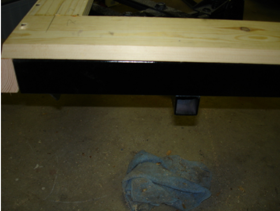
Side table socket welded in place.
