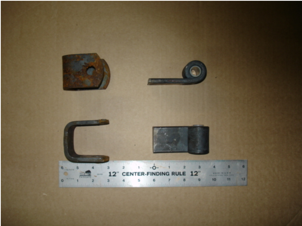
Spring hangers, left side is front hanger, right side with nylon bushing is rear hanger.
