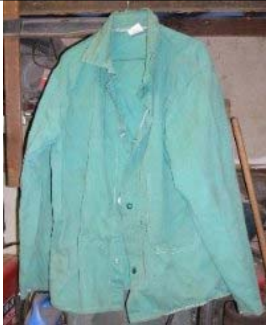
Green welding jacket, handy item to have and it will save you a lot of burns. Much less expensive than the leather sleeves and bib above but a little less burn proof.
