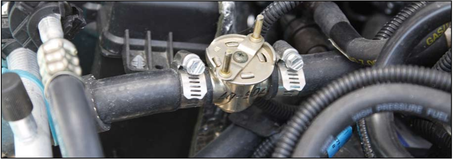
Picture A under hood manual valve location in the Lincoln Town Car
