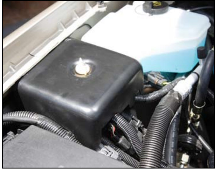
power distribution module with cover on
