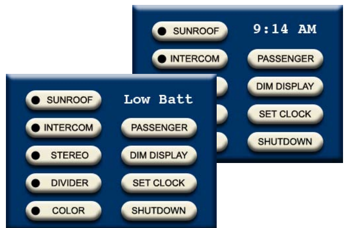
The Clock is replaced by a battery level indicator to notify the driver of a low voltage condition.
