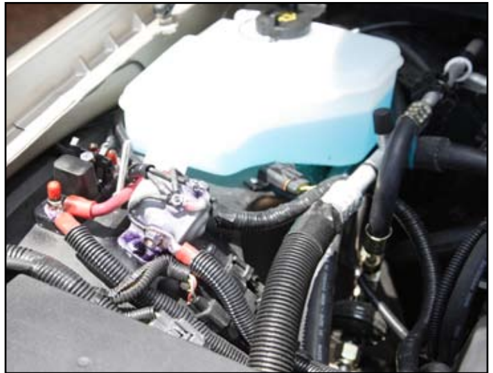
power distribution module with cover removed
