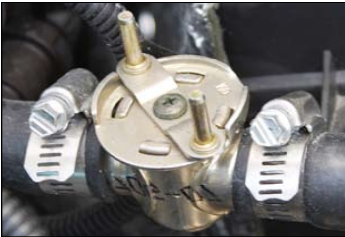
(pic. B) manual valve in off position stops hot water flow
