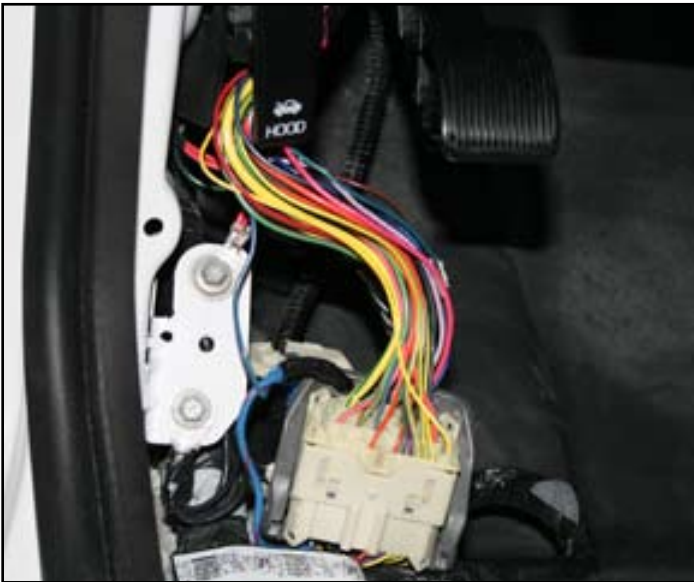
blue/red and blue/light blue wire driver's side A-pillar
