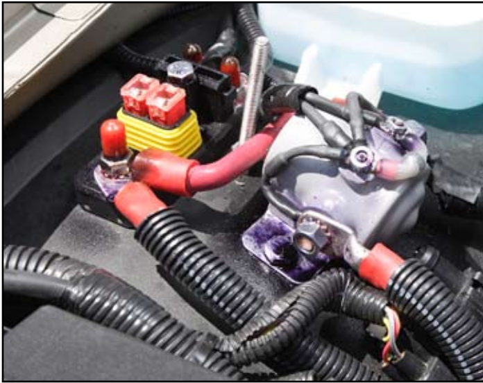
50 AMP Fuse block with fuse cover removed
